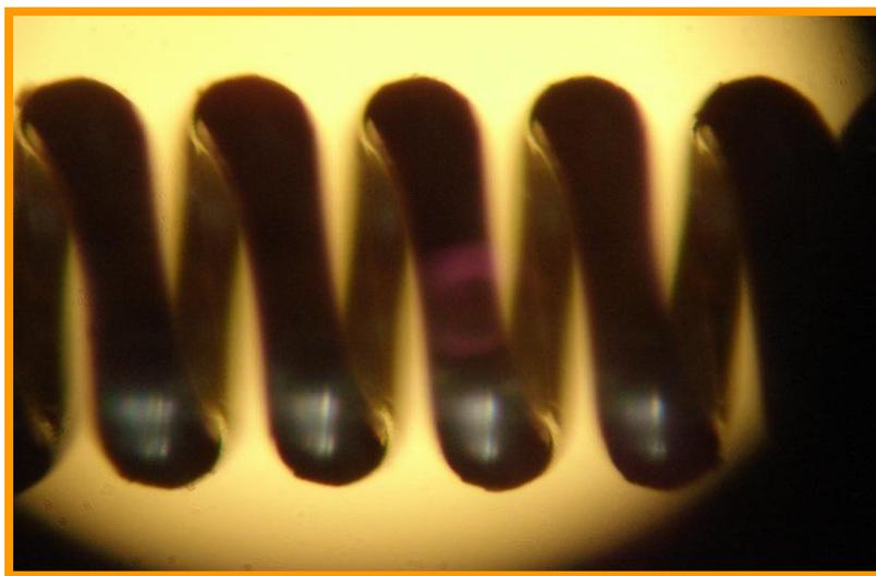
**Figure 7.5.** CWF coated with Apiezon N using low concentration solution (2.5% in  $\text{CH}_2\text{Cl}_2$ ).
